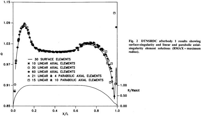
show that it takes a minimum of 45 elements to obtain a good representation of the body and satisfactorily predict the tangential velocity on the body. Increasing the number of surface elements to 70 only goes to improve the representation of the body and the prediction of the tangential velocity. See Fig. 1.
